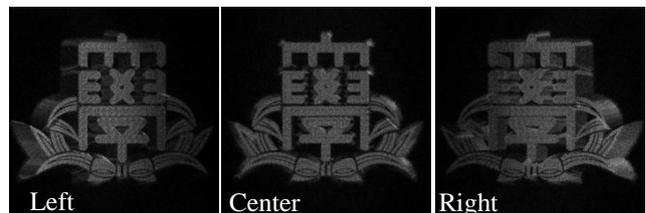
Fig.12 Simulated reconstruction of binary-amplitude Fresnel CGHs encoded by simple threshold.  $z = -100$  mm.
