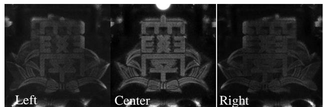
Fig.13 Simulated reconstruction of binary-amplitude image CGHs encoded by simple threshold.  $z = 0$  mm.
