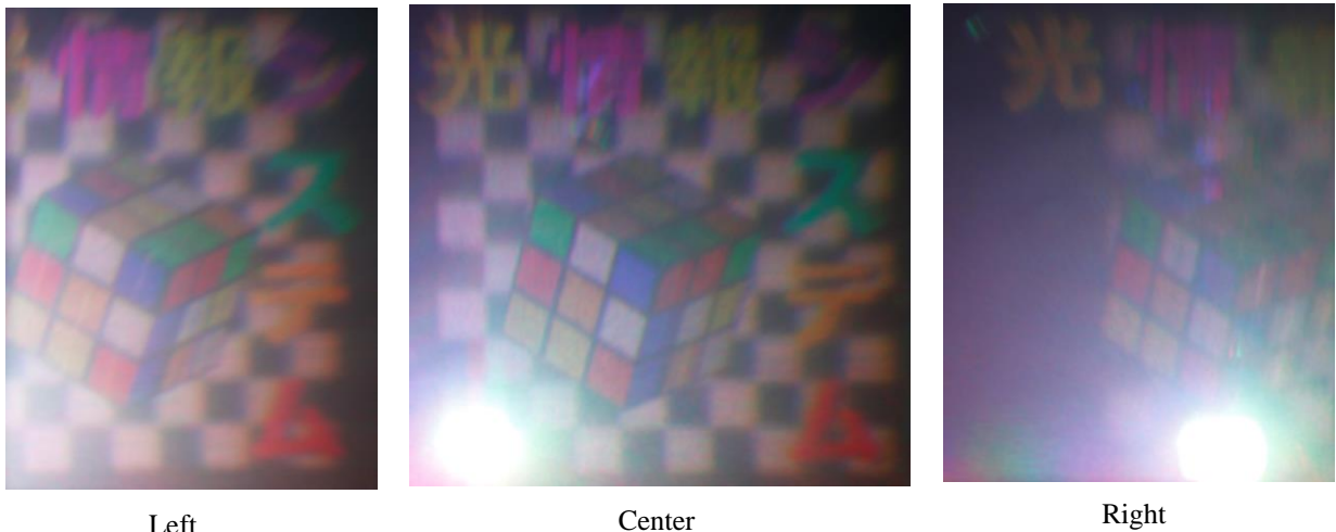
Fig. 10 Optical reconstruction of the full-color high-definition CGH. Pictures are taken from different viewpoints.
