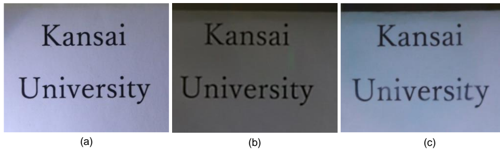
Fig.3 Comparison of transparency between an amplitude CGH and CGVH. (a) A photograph of original printed letters, and photographs of the same letters, but taken through (b) the original amplitude CGH and (c) the transferred CGVH.
