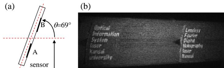
Fig. 9 Numerical reconstruction of planar objects on tilted plane (b) and its procedure (a)
