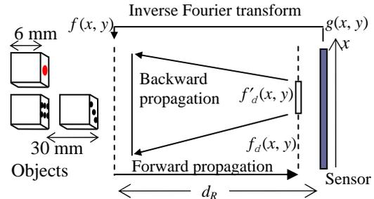
Fig. 5 Procedure for numerical reconstruction from different points of view
