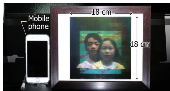
Fig. 2. Optical reconstruction of the full-color sub TPS CGH using RGB color filters [3]. The fringe image is composed of 0.1 T pix.
