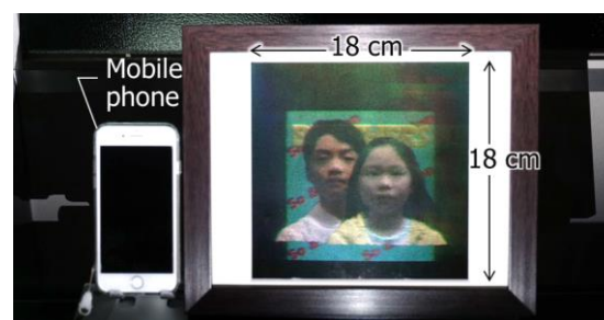
Fig.2 Full-color FPHD-CGH composed of 225,000 \times 450,000 pixels with a pixel pitch of 0.8 \mu\text{m} \times 0.4 \mu\text{m} .
