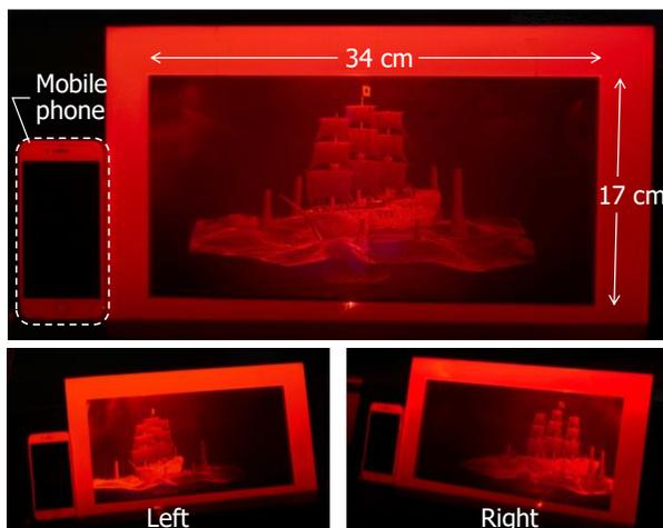
Fig.1 Optical reconstruction of the monochrome FPHD-CGH named Sailing Warship III. The fringe image comprises 425,000  $\times$  425,000 pixels with a pixel pitch of 0.8  $\mu\text{m}$   $\times$  0.4  $\mu\text{m}$ . The illumination light source is a red laser.
