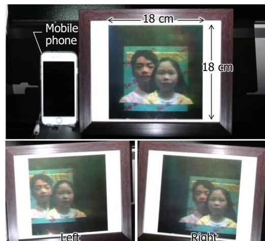
Fig.2 Optical reconstruction of the full-color FPHD-CGH named Color Brothers. The fringe image comprises 225,000  $\times$  450,000 pixels with a pixel pitch of 0.8  $\mu\text{m}$   $\times$  0.4  $\mu\text{m}$ . The illumination light source is an RGB laser.
