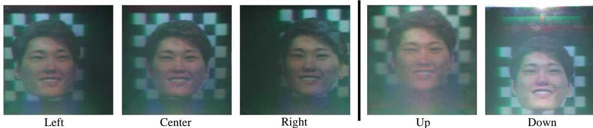
Fig. 3. Closeup photographs of optical reconstruction of the created FPHD-CGH.
