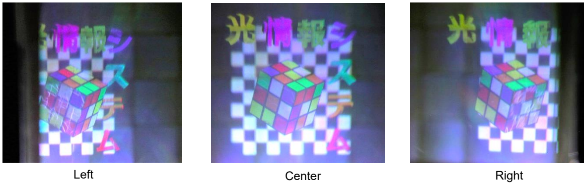
Fig.6 Photographs of optical reconstruction of the stacked CGVH fabricated by tiling contact-copy. The camera is focused on the reconstructed 3D image.
